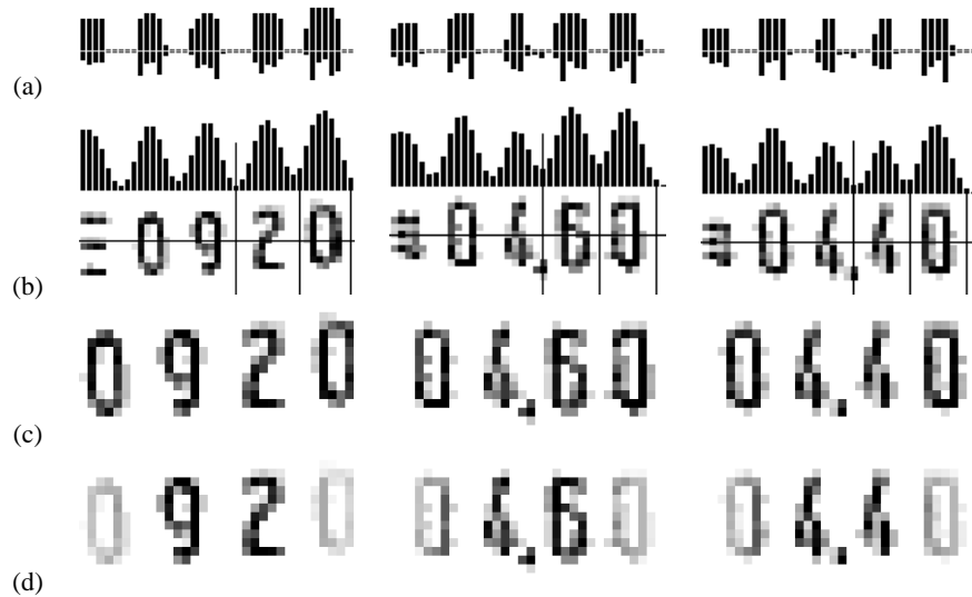
Fig. 7.7. Position normalization. For the examples from Fig. 7.5 are shown: (a) top index (upwards) and column sum (downwards); (b) region of interest with smoothed occupancy index (the start column at the right, as well as two local minima and the vertical center of mass are marked); (c) 32 \times 16 window cut from the region of interest; (d) window with faded borders.
